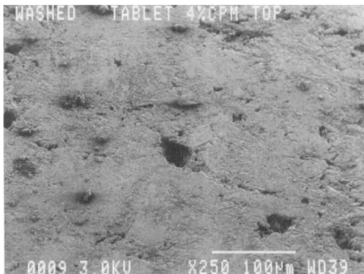
Figure 1. Scanning electron micrograph: tablet immediately after contact with medium.
